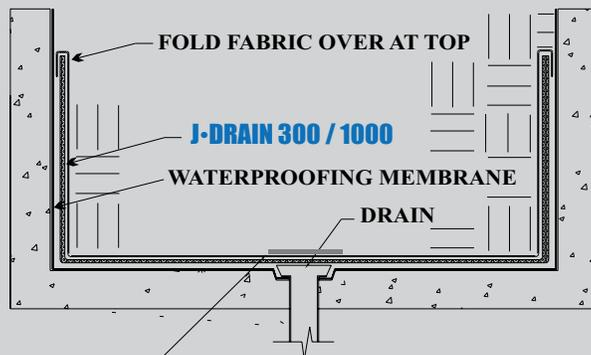
**NOTE:** When using **J-DRAIN 1000**, cut and remove bottom layer of (grey) fabric so water can pass into drain.
