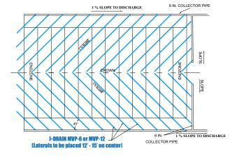
NOTE: J-DRAIN MVP-12 is placed horizontally across playing field and sloped to sideline trenches thus eliminating cross field trenching.
